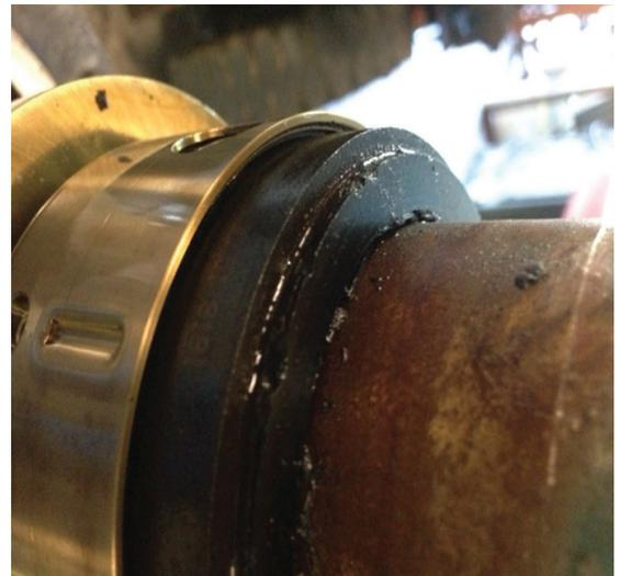
Figure 2. Black Powder contamination on the seals.
