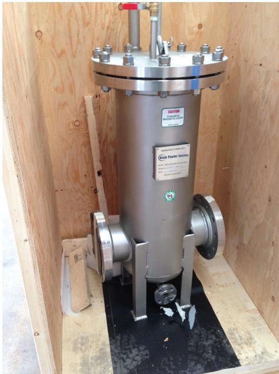
Figure 3. Black Powder Solutions Magnetic Separator
