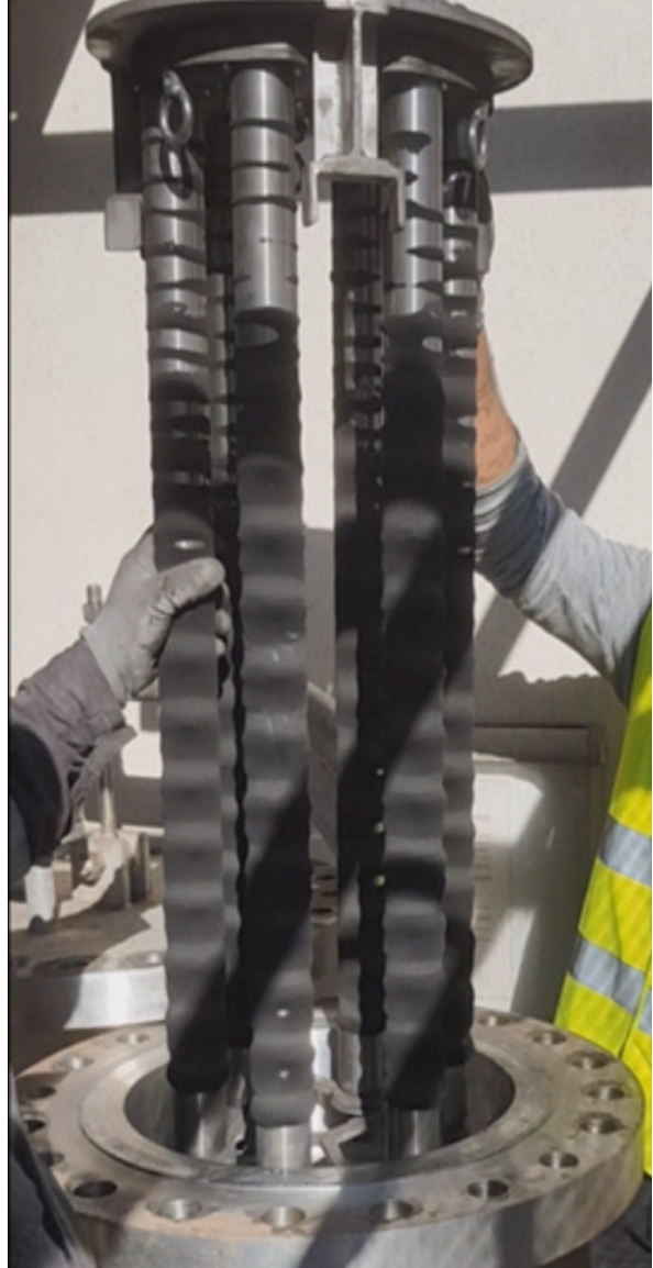
Figure 2. Removing the magnetic array from the magnetic separator for initial cleaning.
