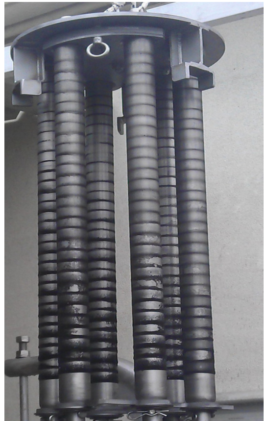
Figure 1. The magnetic array with black powder contamination on it after the array was removed for an initial inspection.
