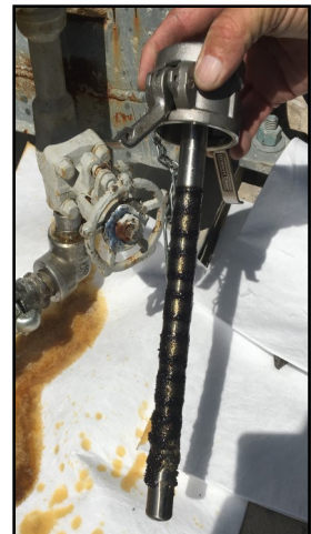
Black Powder contamination captured after 10 minutes.
