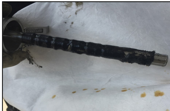
Contamination caught after 1 hour.
