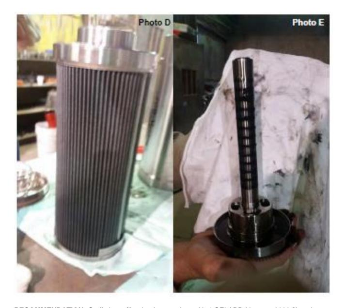
**RECOMMENDATION:** Outfit these filter banks complete with 4 OEI ADD-Vantage 9000 filters in a duplex forma (holding capacity 8+lbs/bank) to extend the cleaning interval even further and protect the compressor. OEI also recommends the installation of a magnetic separator system for the inlet gas to reduce the contamination in the lube oil and protect the compressor and other system components inside the plant.
