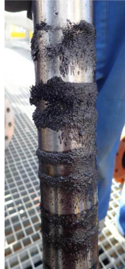
BPS magnetic separator removed for cleaning from VGO feed to the HDS unit.
