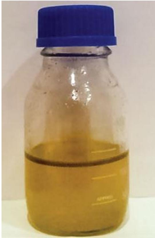
**Fig. 8.** Liquids removed from sour feed gas at HdGP (filter out).
