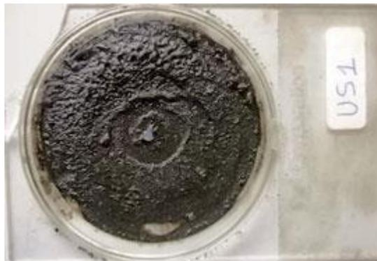
**Fig. 9.** Sludge collected upstream of the cyclone filter near Shedgum.
