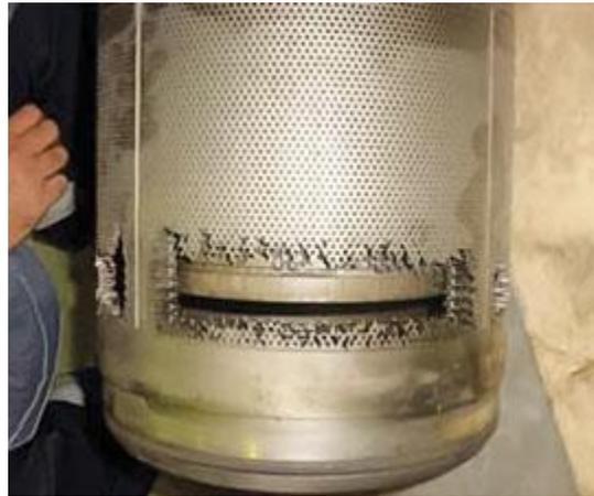
**Fig. 2.** Erosion of a control valve at Berri Junction.
