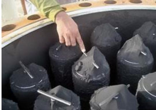
**Fig. 3.** Black powder on absolute filters on sales gas to SAFCO in Jubail.
