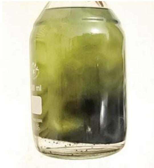
**Fig. 13.** UGP condensate to pipeline (clear layer of water at the bottom).
