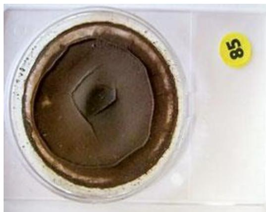
**Fig. 7.** Solids removed at sour feed gas at ShGP.
