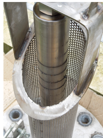
Analysis of the contamination collected indicated high levels of non-ferrous particulate caught by the magnetic elements
